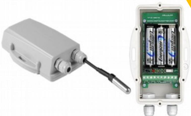
**PQ - FALCON Cellular is a super smart, battery powered monitoring device in a rugged housing. Super long battery life is possible with LTC (Lithium Thionyl Chloride) batteries, or connect to a power source for a permanent solution.**
